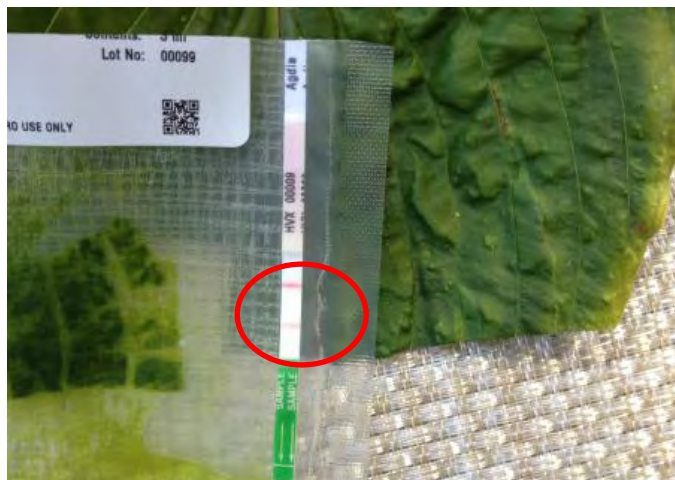
Second line (below control line) shows this hosta is infected with HVX
