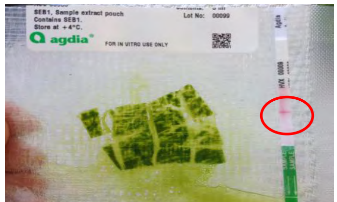
Control line on the test strip proves it is working properly
